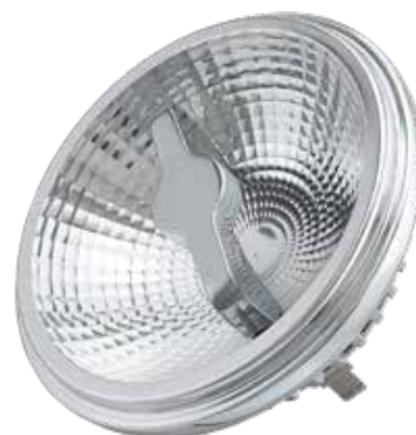
PLC-50719 Ambient Dimming Reflector AR 111 15 W / 650 lm / 2000 - 3000 K incl compact driver
